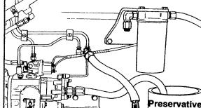
Drain the preservative oil from the lubricating oil pan and the oil filters. Install the drain plug.
