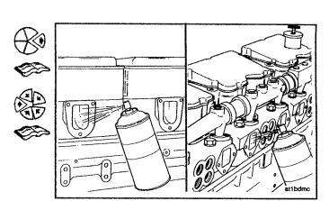
Remove the rocker housing covers, and spray the rocker levers, crossheads, valve springs, valve stems, valve guides, and the push rods with preservative oil. Install the rocker housing cover.
