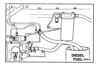
Flush the fuel system with clean diesel fuel to remove preservative oil.
