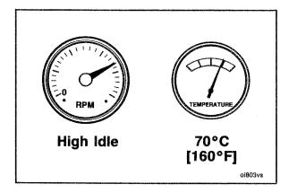
Operate the engine at the high idle throttle position until the coolant temperature is 70°C [160°F].
